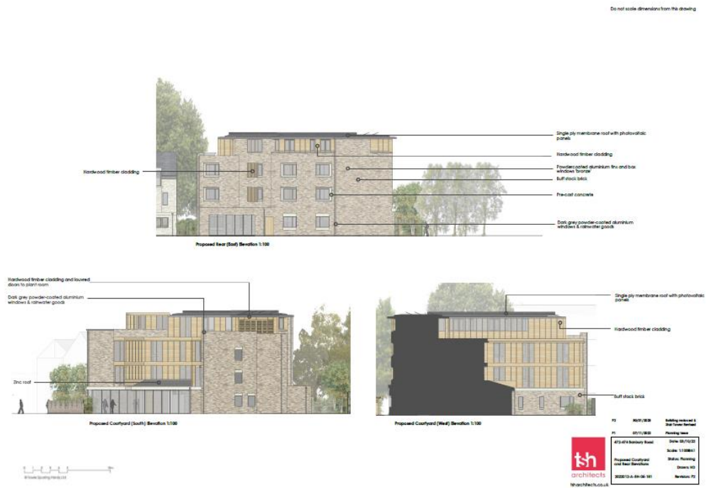
Figure 3: East and courtyard elevations
